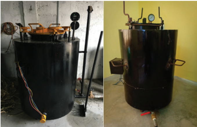
High pressurized electric boiler developed for cooking lokta bark.
