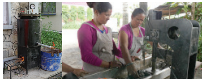
Cooking and beating system for refining Allo and Washing system for refining Allo
