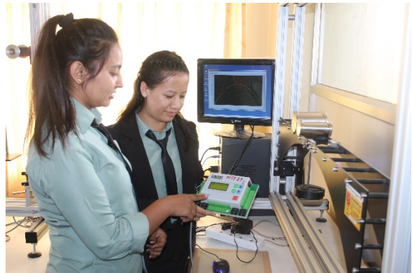
Three hinged arch (Structure lab)
