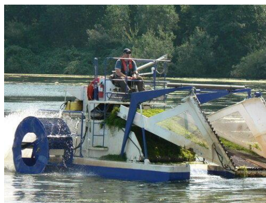
Figure 9: Hyacinths extraction using mechanical harvester [21].
